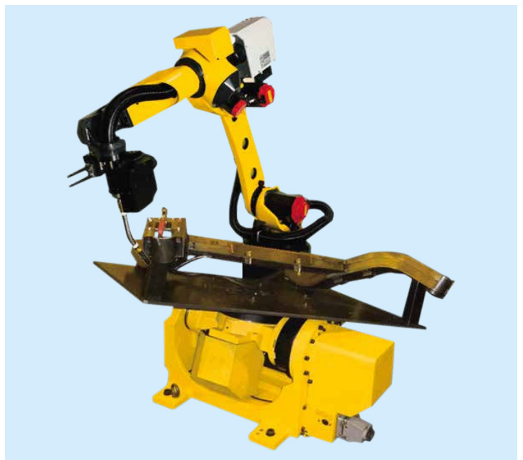
Automobile part arc welding with 2-axis positioner
