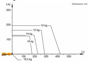
The KR 16 R2010 is designed for a rated payload of 16 kg in order to optimize the dynamic performance of the robot. With reduced load center distances and favorable supplementary loads, a maximum payload of up to 19.2 kg can be mounted. The specific KUKA Load case must be verified using KUKA. For further consultation, please contact KUKA Service.
