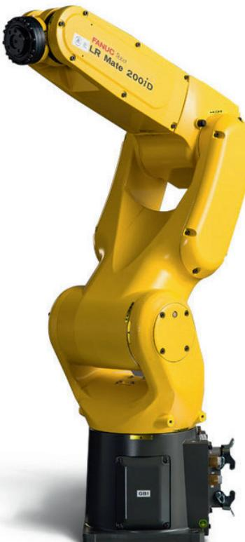
Standard model (2 integrated solenoid valves)
